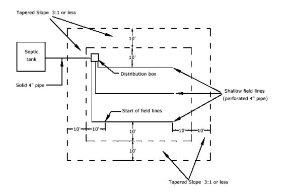
Capping Fill System - Top View (6% - 12% Slope)
