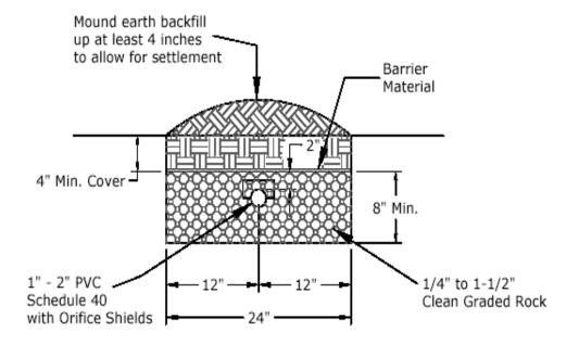
Capping Fill System - Top View (Less Than 6% Slope)
