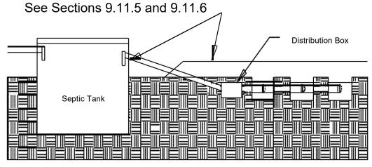
Note: Capping material must extend 10 ft. from trenches before the start of the slope. The tapered slope shall be 3:1 or less.
