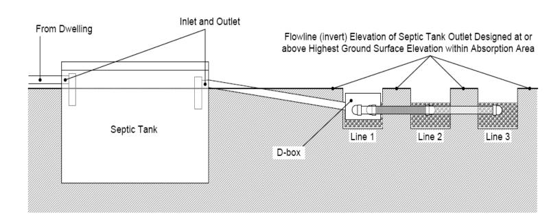
• The slope across the drain field starting from the first line to the last line is < 6 inches.
