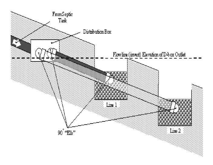
• Elevation change from the first line to last line is  $\geq 6$  inches.
