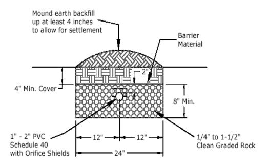
Capping Fill System - Top View
