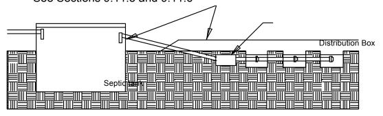
Note: Capping material must extend 10 ft. from trenches before the start of the slope. The tapered slope shall be 3:1 or less.
