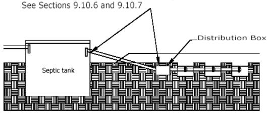
Note: Capping material must extend 10 ft. from trenches before the start of the slope. The tapered slope shall be 3:1 or less.
