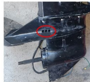
MODIFIED OUTBOARD EXHAUST
